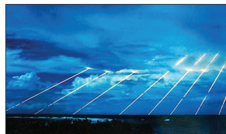
A W87 is part of the ICBM “leg” of the nuclear deterrence triad. This is a time-exposure shot of eight W87 Peacekeeper reentry vehicles launched from a single missile. The Air Force refers to these as reentry vehicles (RVs); the Navy refers to them as reentry bodies (RBs).
